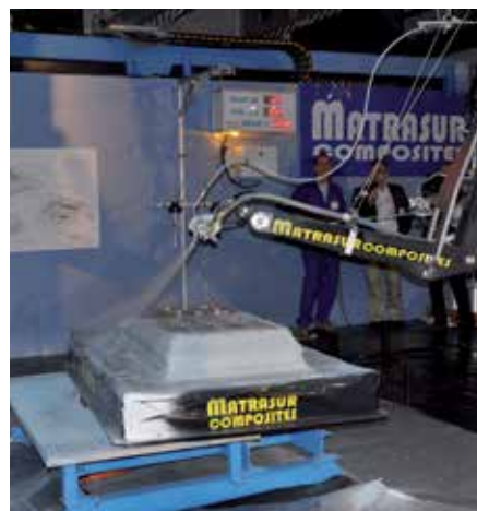
10-axes spray-up robot type ROBOTAT for gelcoat and resin & fiberglass in action
