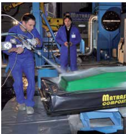
Instantaneous programming based on the copy of the operator's movements by the robot
