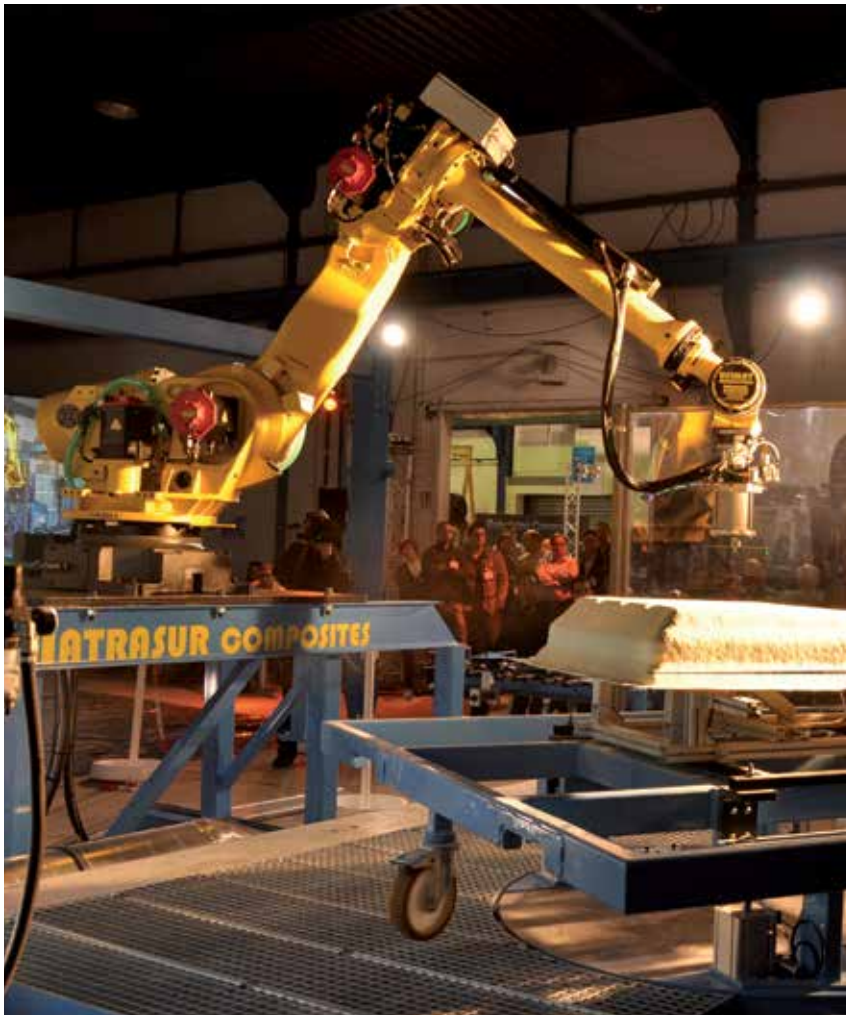
7-axes trimming robot type USIMAT in action
