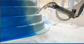
Multi-colour gelcoat spray-up at around 6 m<sup>2</sup>/min
