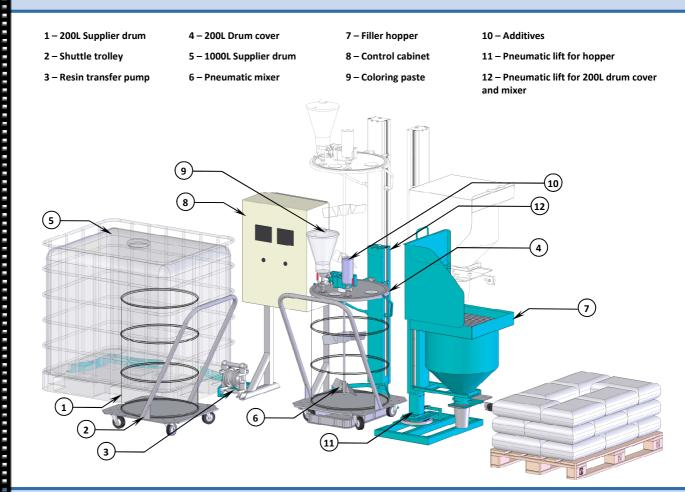
Mixing station for resin and fillers Simple, efficient, secured, and economic
