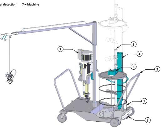
Continuous material supply of mobile machine by means of a shuttle trolley for supplier drum of 200L
