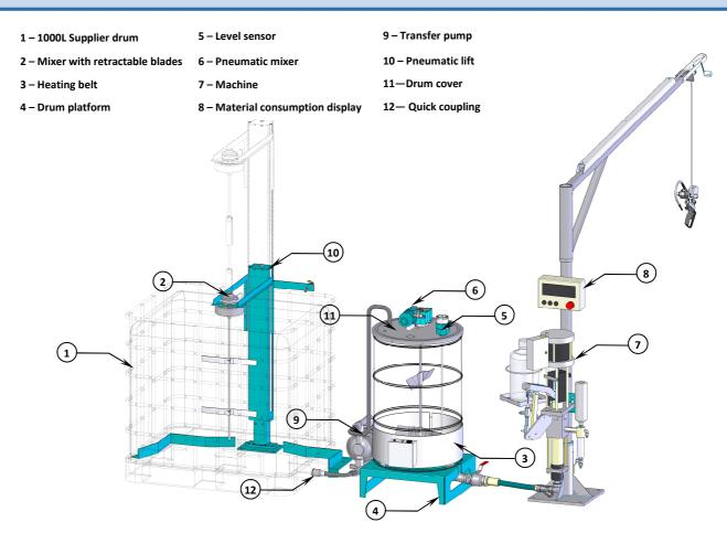
Continuous material supply of machine buffer drum by means of a supplier drum of 1000L
