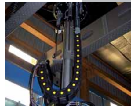
Robot's vertical axis (1.60 m - 5.25 ft) Axe verticale du robot (1,60 m)
