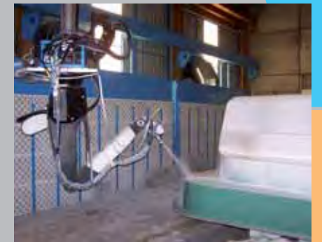
Gelcoat spray-up (6m² - 65 ft²/min) Projection gelcoat (6m²/min)
