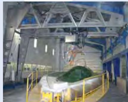
Gelcoat spray-up on a complex-shape mould Projection gelcoat sur moule aux formes complexes
